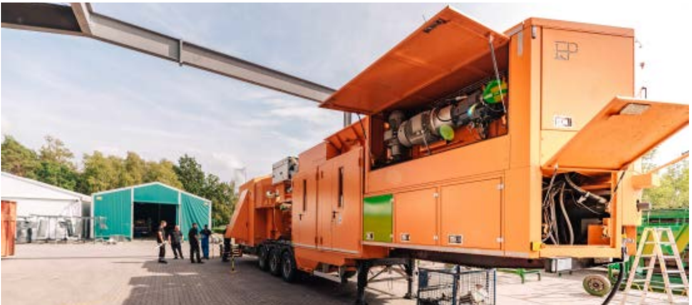
Trailer-mobile channel baler – enclosed and sealed to prevent fibre fly.
